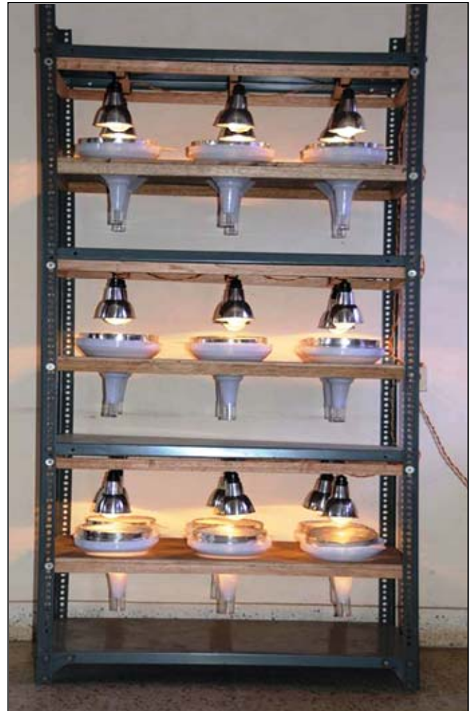
Fig. 5: Fabricated a low cost Berlese-Tullgren Funnels extractor in laboratory
